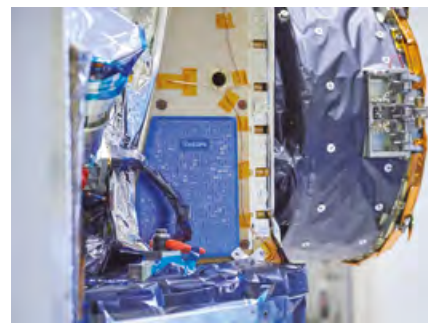
The two titanium plates attached to Cheops
